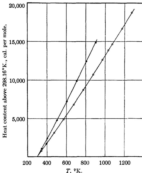
Fig. 1.—High temperature heat content of vanadium chlorides: upper curve, VCl<sub>3</sub>; lower curve, VCl<sub>2</sub>.
